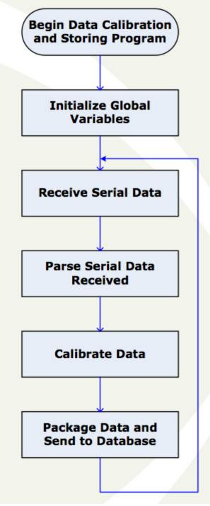
Figure 45: Python Code Calibration and Storage Flow Chart
