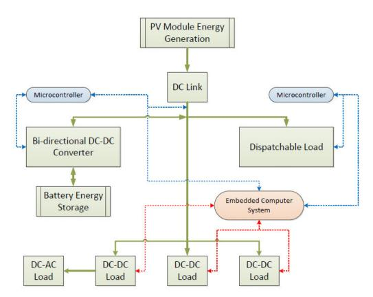
Figure 5: Initial Projected Block Diagram of DC Microgrid
