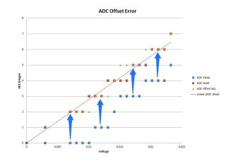
Figure 63: ADC Offset Error
