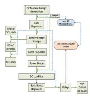
Figure 36: Hardware Block Diagram Model
