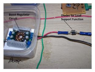
Figure 41: Boost Regulator installed on prototype and interfaced with diodes
