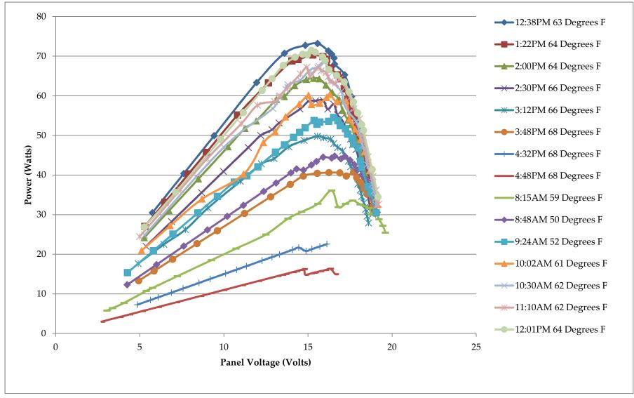
Figure 59: Ramsond 100W Mono-Crystalline Power Output versus Panel Voltage
