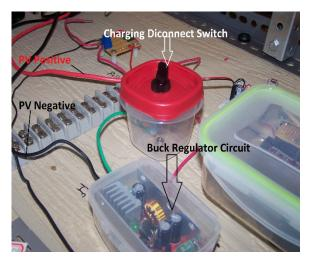
Figure 39: Buck Regulator interfaced with Disconnect Switch (in on position)
