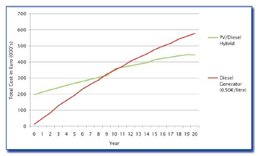
Figure 27: Cost over time of PV microgrids and Diesel microgrids. Courtesy of <u>http://www.ruralelec.org</u>
